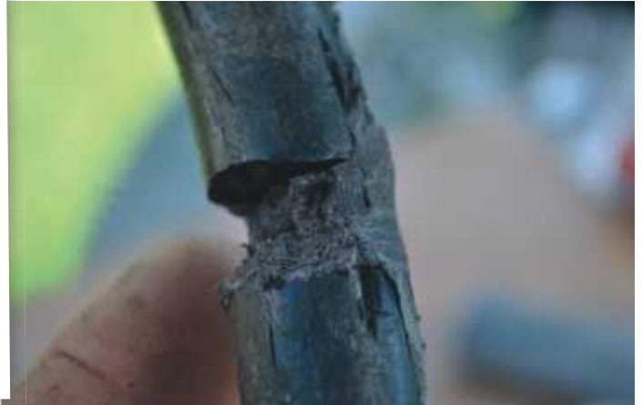
12 The main crack needed more putty than I first anticipated so a second mix was required.
