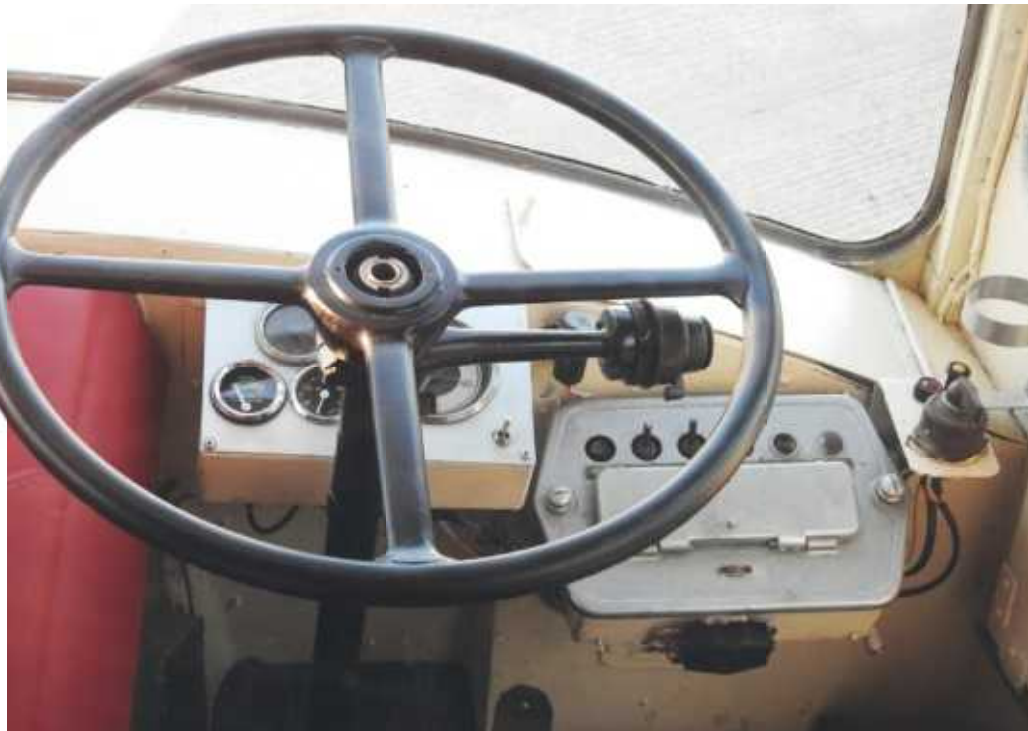
▲ After the first outings, a larger steering wheel was fitted to reduce effort negotiating sharp turns and roundabouts.
