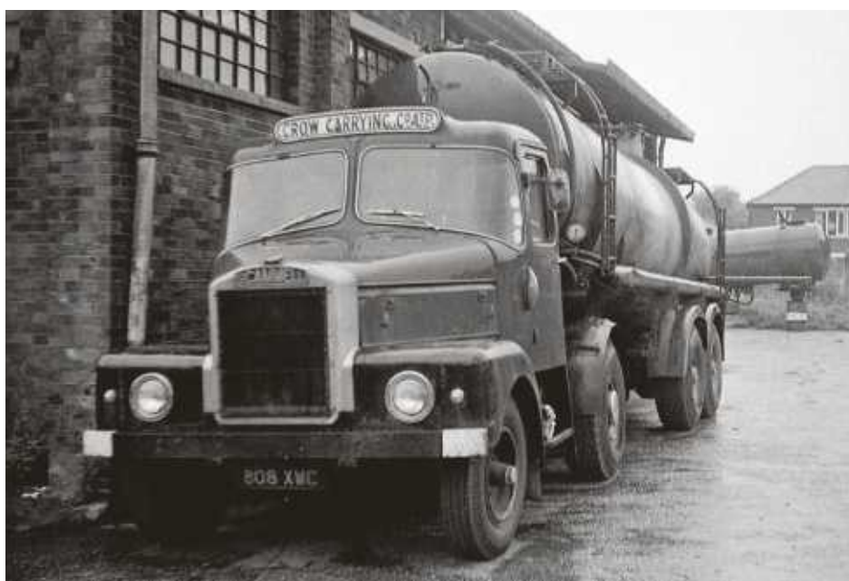
▲ Crow Carrying Co was still putting new Scammell Highwayman tractor units into service with matching tank trailers in the 1960s, like 808 XWC (Essex, 1963). Another Scammell tank trailer, separated from its unit, can be seen to the rear, its front coupling propped up on a barrel as there were no landing legs fitted.
