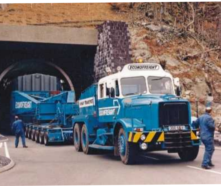
Photos above & right: Mike Hetherington recalls this job into Dinorwic in North Wales was in 1986 and involved a 260 tonnes transformer: "The skirt and ducting had to be fitted after the trailer had negotiated the tunnel as the clearance was very tight. I remember Albert Vincent telling me one of the lads was standing in the goosenecks to watch the clearance and got a face full of bats which were hanging off the tunnel roof." Mike recalls the Series 2 equipment wasn't as good as 1 in service so wasn't used.
