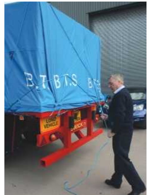
▲ Dennis adjusting the ropes around the back of the load to make them tighter. You'll have to ask him why this arrangement is called 'Scotchman.'
