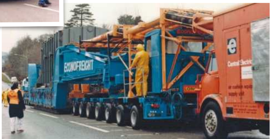
Photos above & right: Mike Hetherington recalls this job into Dinorwic in North Wales was in 1986 and involved a 260 tonnes transformer: "The skirt and ducting had to be fitted after the trailer had negotiated the tunnel as the clearance was very tight. I remember Albert Vincent telling me one of the lads was standing in the goosenecks to watch the clearance and got a face full of bats which were hanging off the tunnel roof." Mike recalls the Series 2 equipment wasn't as good as 1 in service so wasn't used.
