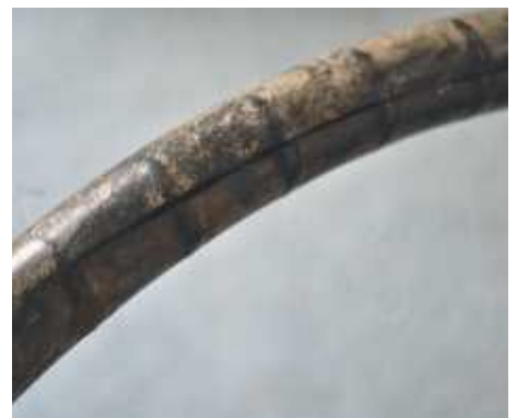
4 Another age-related crack on the underside of the steering wheel.
