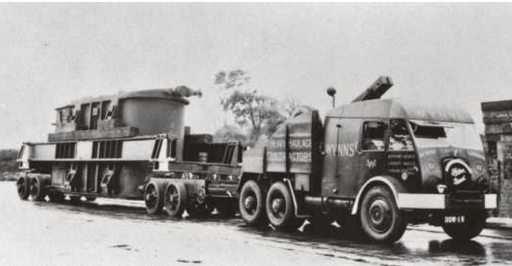
Above & below: Both Wynns and Pickfords show off how to make their own style of girder trailers. The Wynns set-up dates from 1943 and had a capacity of 90 tons. It is seen in 1948 headed up by a special 6x4 Foden 100 tonner.
