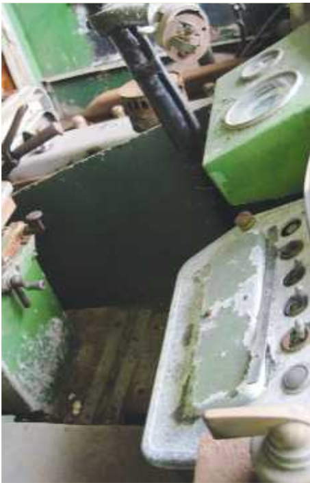
▲ Prudent upgrades included supplementing the original vacuum gauge and speedo with oil and water gauges.
