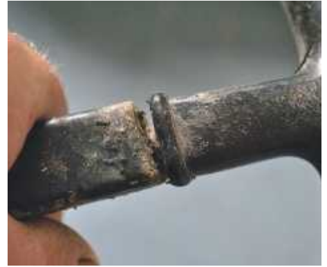
2 A typical shrinkage crack where the metal centre meets the plastic.
