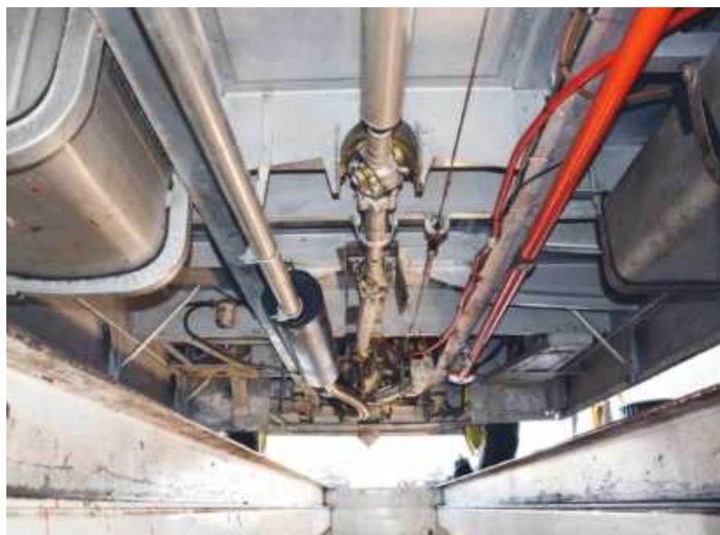
◀ Dartford, Kent bus and coach builder Beadle used an all-aluminium underframe instead of a conventional chassis.
