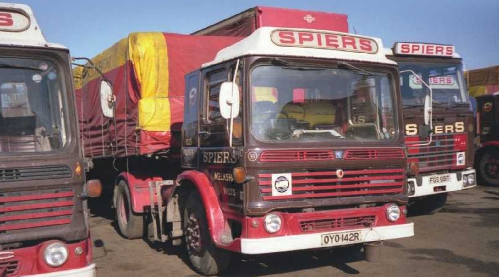
▼ Spiers of Melksham became known for running a fleet of AEC Mandator artichoke units, rebuilt with sleeper cab extensions, on long distance general haulage, like ex-Amoco fleet no 35, OYO 142R, lined up in the yard with others, with a neatly roped and sheeted load on its platform trailer.
