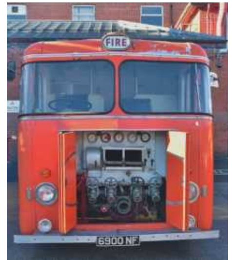
▲ Although it was a capable vehicle in many respects, fire brigades were wary of ordering the Firemaster. The appliance carried a front mounted pump behind hinged doors, where you would normally expect to find a radiator. This was too radical for many fire chiefs.
