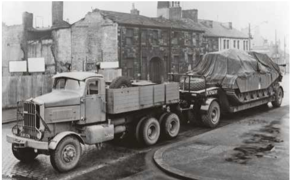
▲ Known as a float trailer (as it floated behind) this Crane drawbar low loader was rated for 60 ton loads. And while back then each 4-in-line was considered as being of two axles, in essence up to 40 tons a row could pass through onto the road surface.
