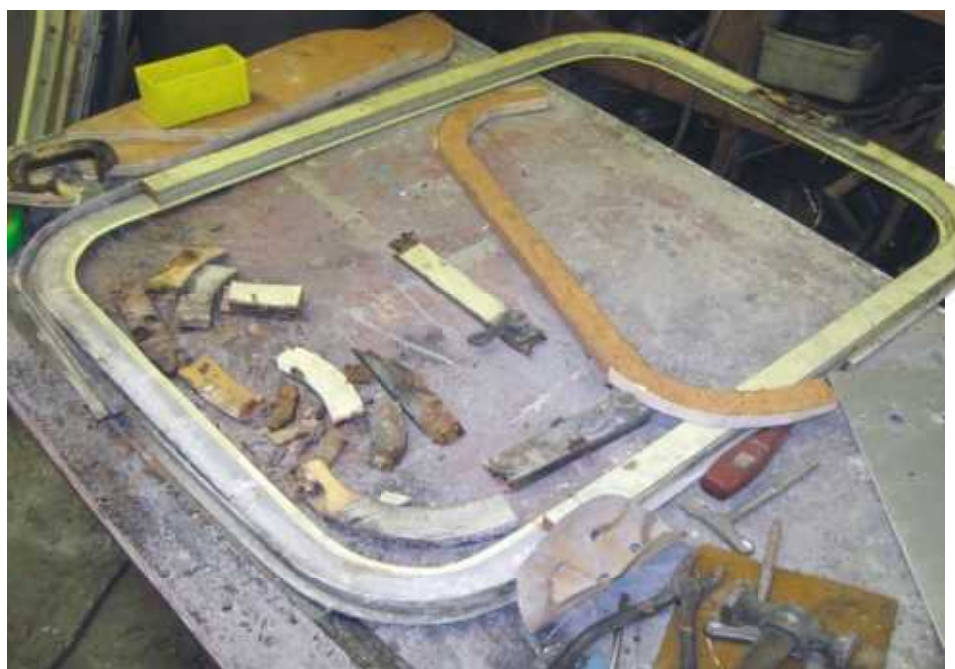
▲ Ray Walsh's self-taught coachbuilding skills came into their own making new frames and wooden panelling.
