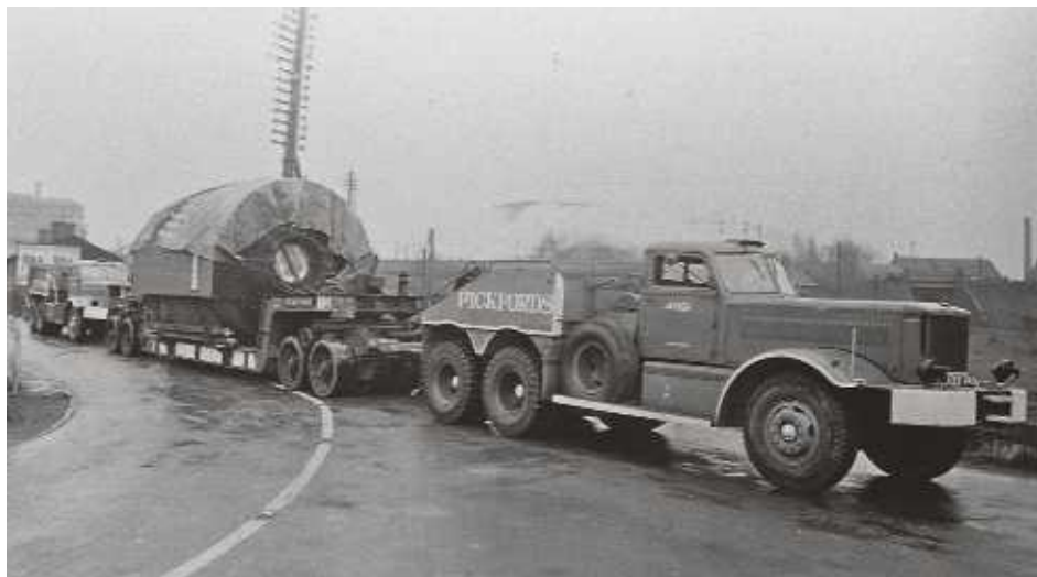
▲ Pickfords were given dispensation to buy these Diamond T 980s during the war years. This was the strongest type of 'girder' trailer they had for work at this time and was rated for 140 ton loads.
