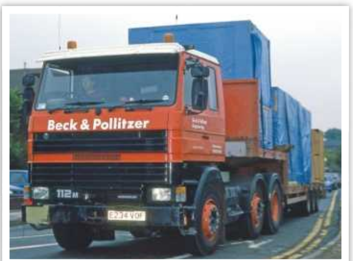
▲ Beck and Pollitzer have long specialised in heavy haulage and machine installation. They have used a variety of tractors including Scania 141 V8s, and in July 1994 I captured this twin-steer 112 and loaded step frame trailer from the Midlands division of the company.
