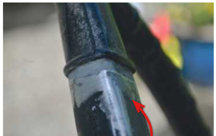
14 Once hard it can be sanded back to the correct profile.
