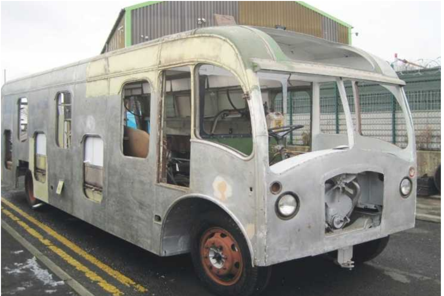
▲ By the middle of last winter, the Beadle bodywork had been made good and ready for painting, which took two weeks.
