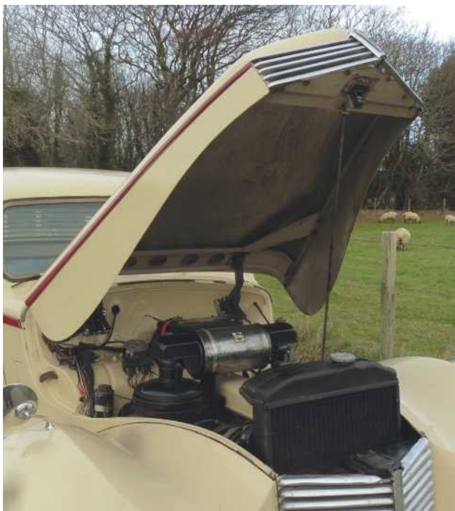
▲ The alligator-style bonnet as fitted to many cars of this period.
