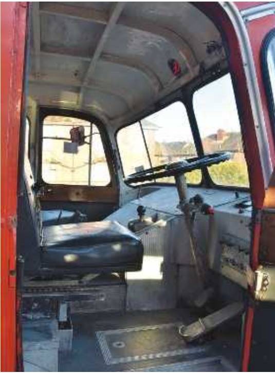
▲ The Firemaster's cab. Appliances of this era lacked driver friendly equipment, like a synchromesh gearbox and power steering.
