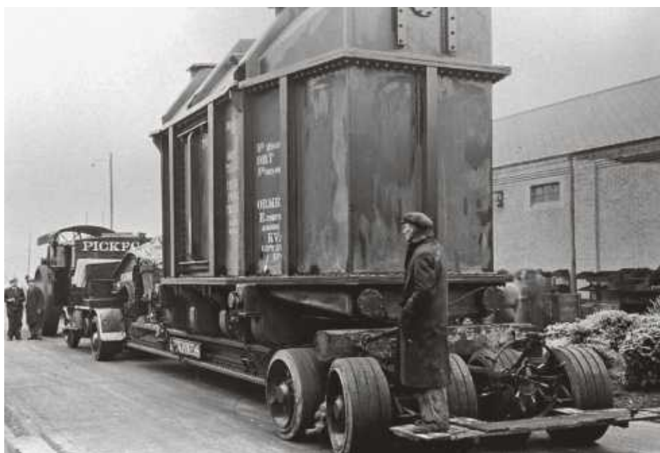
▲ The first Scammell 100 tonner, and while it's not a girder trailer outfit, the semi-trailer is built in girder fashion. Originally there was a small hut on the back but over time, this was removed and the trailer man had to contend with the elements.
